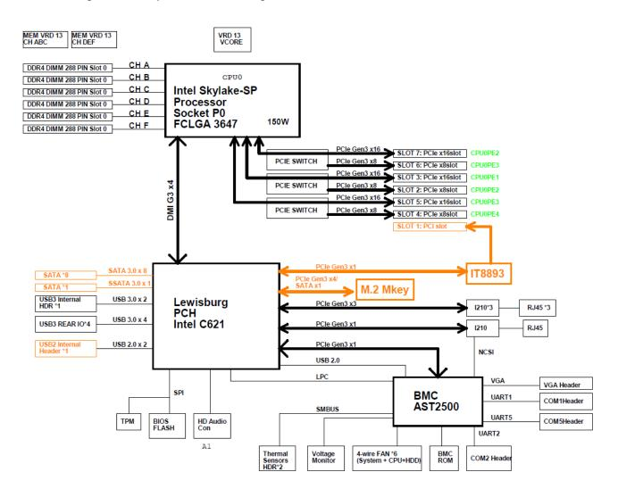
Figure 1-1 System block diagram
