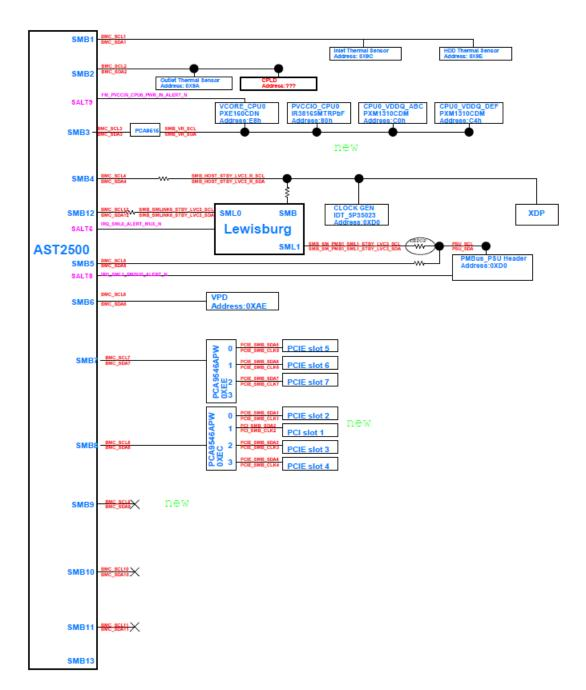
Figure 1-2 I2c block diagram
